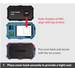
and secure with the six screws. partition and formatted using the OS before using. If the SSD/HDD have existing data, the file manager should be able to see your files.
