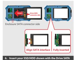
connector facing up all the way into the Enclosure SATA connector. Make sure the SATA connectors seats securely into each other.
